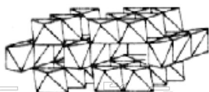
(a) 1x1/1x2 tunnel intergrowth (nsutite)
